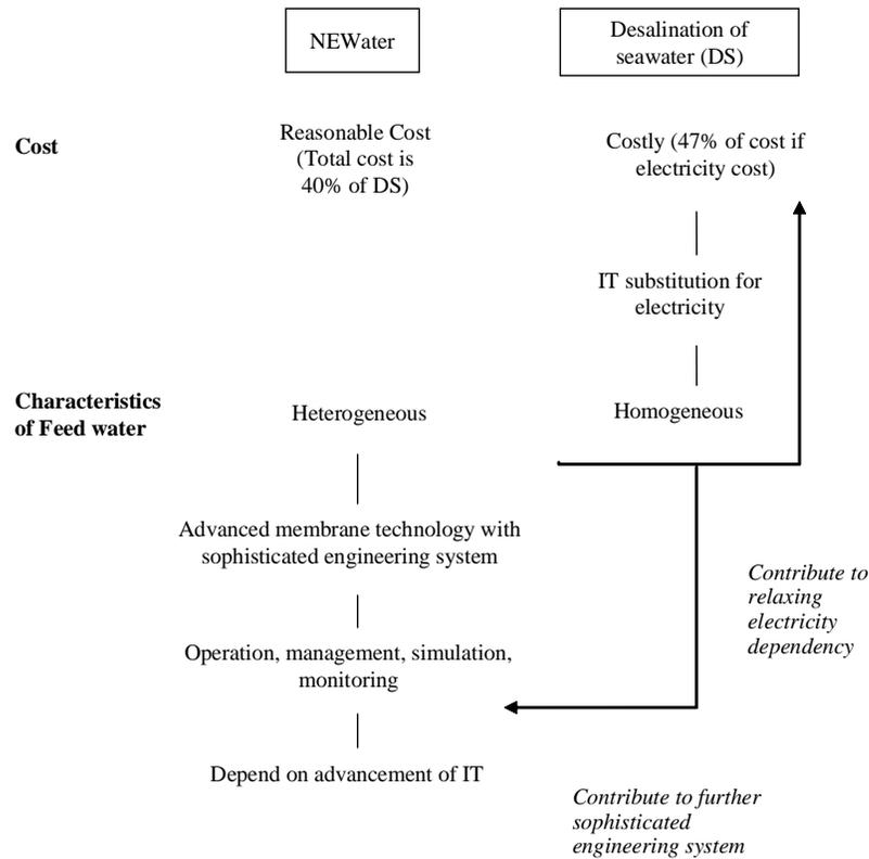
Figure 2: Complementary Relationship between NEWater and Desalination
